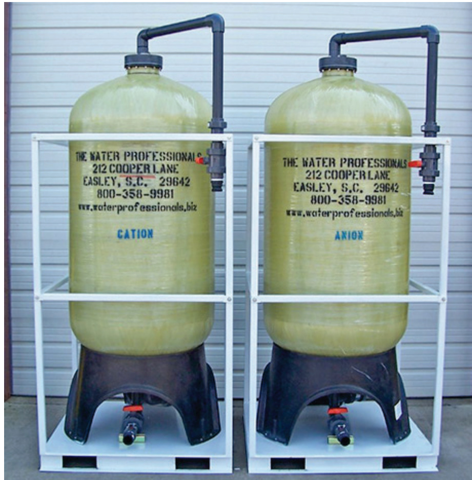
Kation exchange: AmberLite HPR1200 H Anion Exchange: HPR4100 Cl
