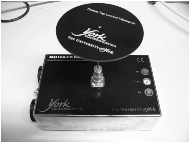
Fig. 8. Noise emitter CNEIII with the 100-mm top-loaded monopole antenna.
