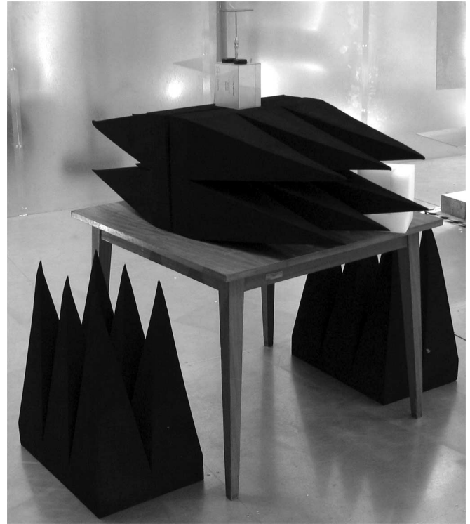
Fig. 15. Comb generator RSG2000 with four blocks of absorbers to simulate an EUT with a higher chamber loading. A different loading was realized by using only the two absorber blocks on the table.
