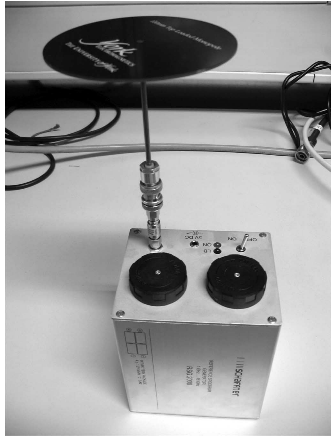
Fig. 9. Comb generator RSG2000 with the 100-mm top-loaded monopole antenna.
