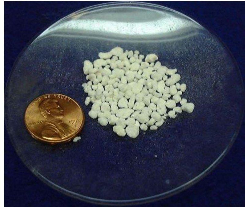
Perlite (volcanic glass) with white, powdery appearance
